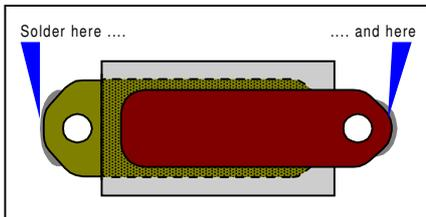
**Fig 22: PCB plate construction viewed from below. The critical parameters are:- 1) the plate corners are arbitrarily radiused, 2) the dielectric is larger than the plate overlap zone by at least 3mm in all dimensions, 3) the cut edges of the plates are rubbed smooth and 4) the plates are different widths so that the long edges are not aligned. Thereafter, the absolute size and shape of the plates is completely unimportant.**
