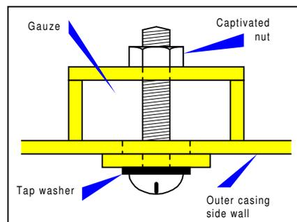
**Fig 19: Suggested silica gel chamber construction - approx 25 x 12mm - made from polystyrene with nylon gauze bonded over the two open sides. The nut is bonded with epoxy resin to captivate it (liberally grease thread with DC4 first). The access hole in the casing is about 5mm and is sealed with an external polystyrene 'washer' and some bathroom sealant. The screw is sealed with a tap washer.**
