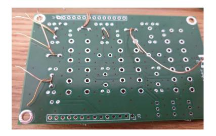
After all Toroids are Placed and soldered, it should look like next Photo. You can also guess what's next.... Place and solder Jumper Connectors, SMA Jack and PA FET's.
