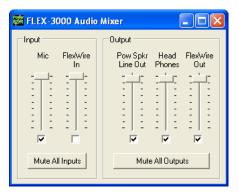
Check *Mic* as the Input to select the front *Microphone* jack. Check *Pow Spkr Line Out* as the Output, to select your powered speakers. Check *Head Phones* if you instead (or simultaneously) want to send audio to the front *Phones* jack.
