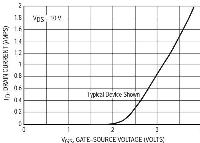
Figure 5. Drain Current versus Gate Voltage
