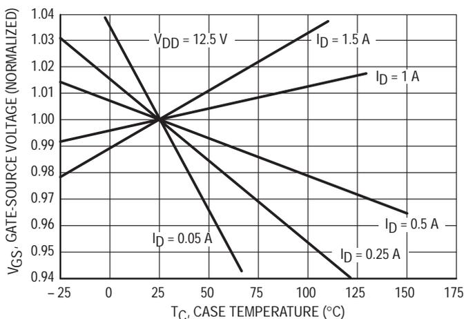
Figure 7. Gate-Source Voltage versus Case Temperature
