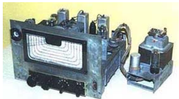
"PTS-47". Built-in broadcasting receiver. Model 1947.
